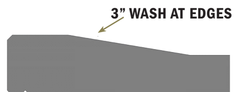
Slope the slab to interior drains and provide a 3-inch wash around all edges.
