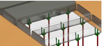
Most longforms are made to create six-inch joists between voids but accommodations can be made for wider joists, if necessary. Because they are one-piece pans, there is little flexibility in changing the void layout from floor to floor or bay to bay. For economy, the pan layout needs to be consistent throughout the structure. However, an efficient layout using this system often results in substantial formwork savings and therefore, lower structure costs.
